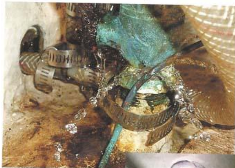
The through-hull valve shown here (above) has been eaten by electrolysis and is leaking, putting the boat in immediate danger of sinking. The other photo (right) shows a professionally bonded through-hull connection.
